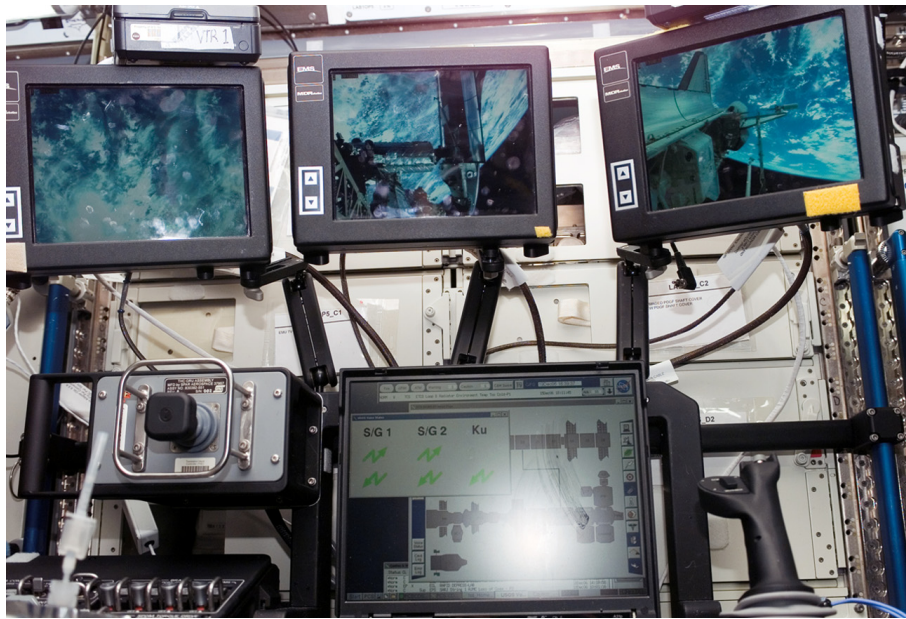
Fig. 1. Robotic Workstation (RWS) used on the ISS. The three monitors of the RWS have three different camera views of the workspace and target payloads. The two laptops mounted above the RWS displays show two additional camera views. Photo credit: NASA.
